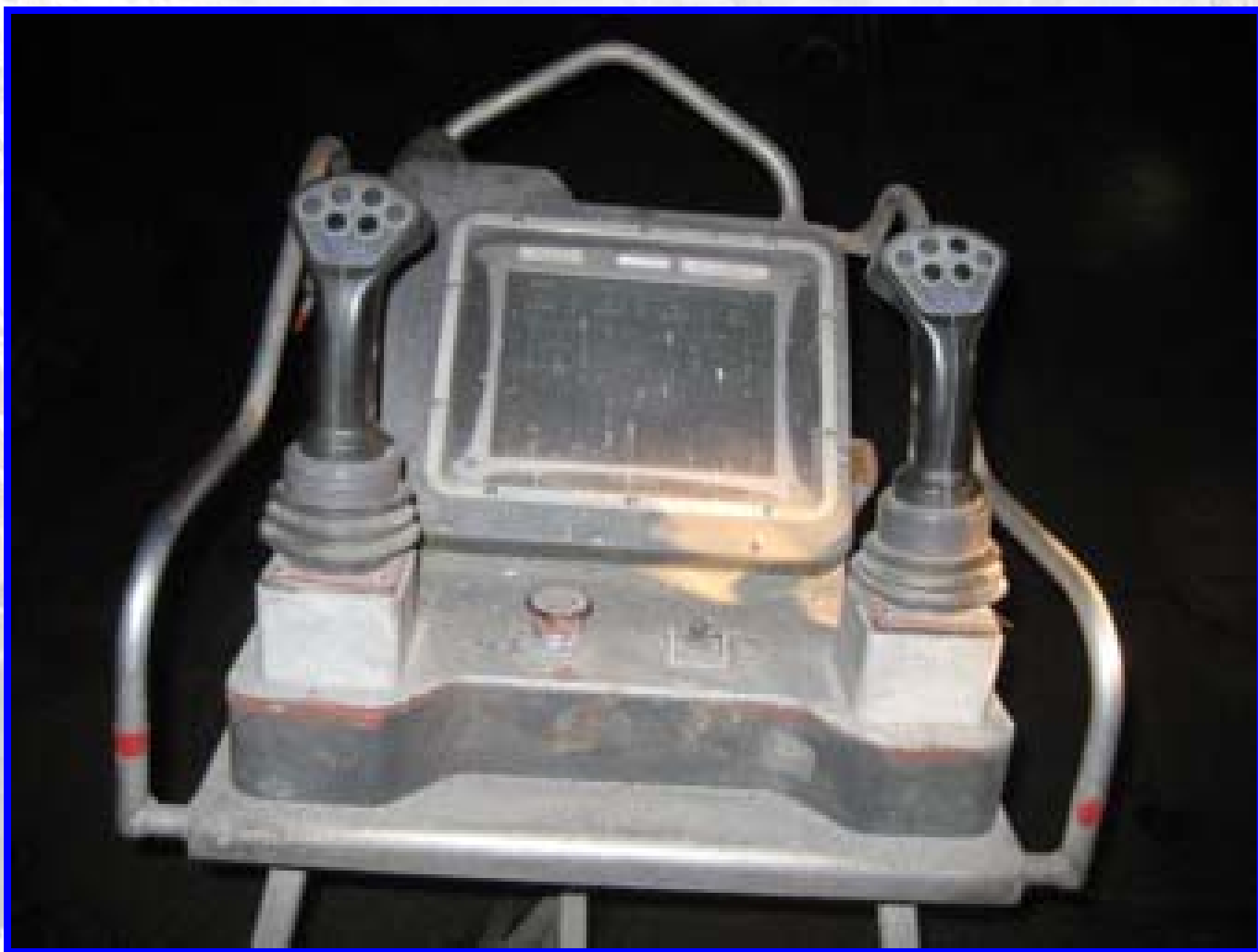
Close-up of the control panel on the “Jumbo” drill, underground at Duck Pond
