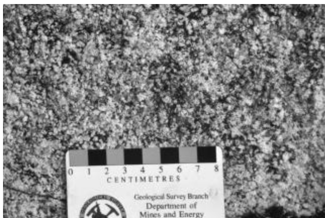
Plate 2. Typical field aspects of white-weathering, medium-grained and massive orthopyroxene-bearing diatexite (granodiorite; Sample 2).
