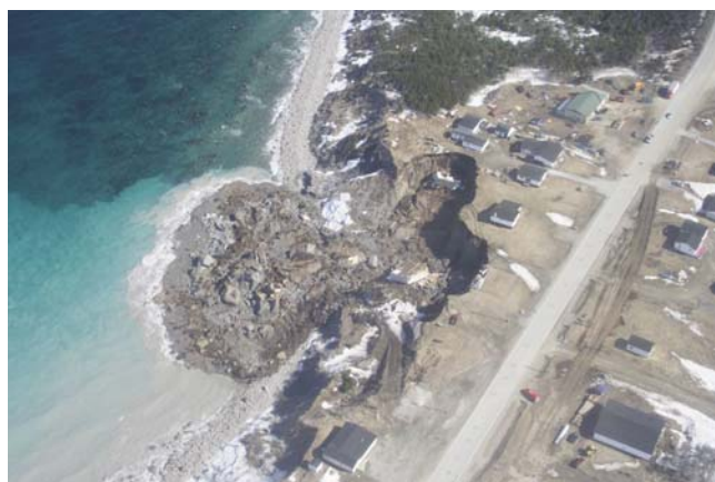
Plate 2. Daniel's Harbour following the 2007 landslide. The slide resulted in the destruction of several houses, relocation of residents and removal of property within the landslide hazard zone, and led to the moving of the Northern Peninsula highway farther inland. Although this disaster is unrelated to rising sea level, it is reasonable to expect that the frequency of such incidents will increase with rising sea levels.
