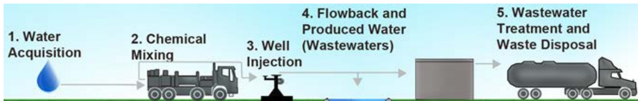
Figure 6: Water cycle in hydraulic fracturing; from U.S. EPA's Study of the Potential Impacts of Hydraulic Fracturing on Drinking Water Resources, Progress Report, 2012.
