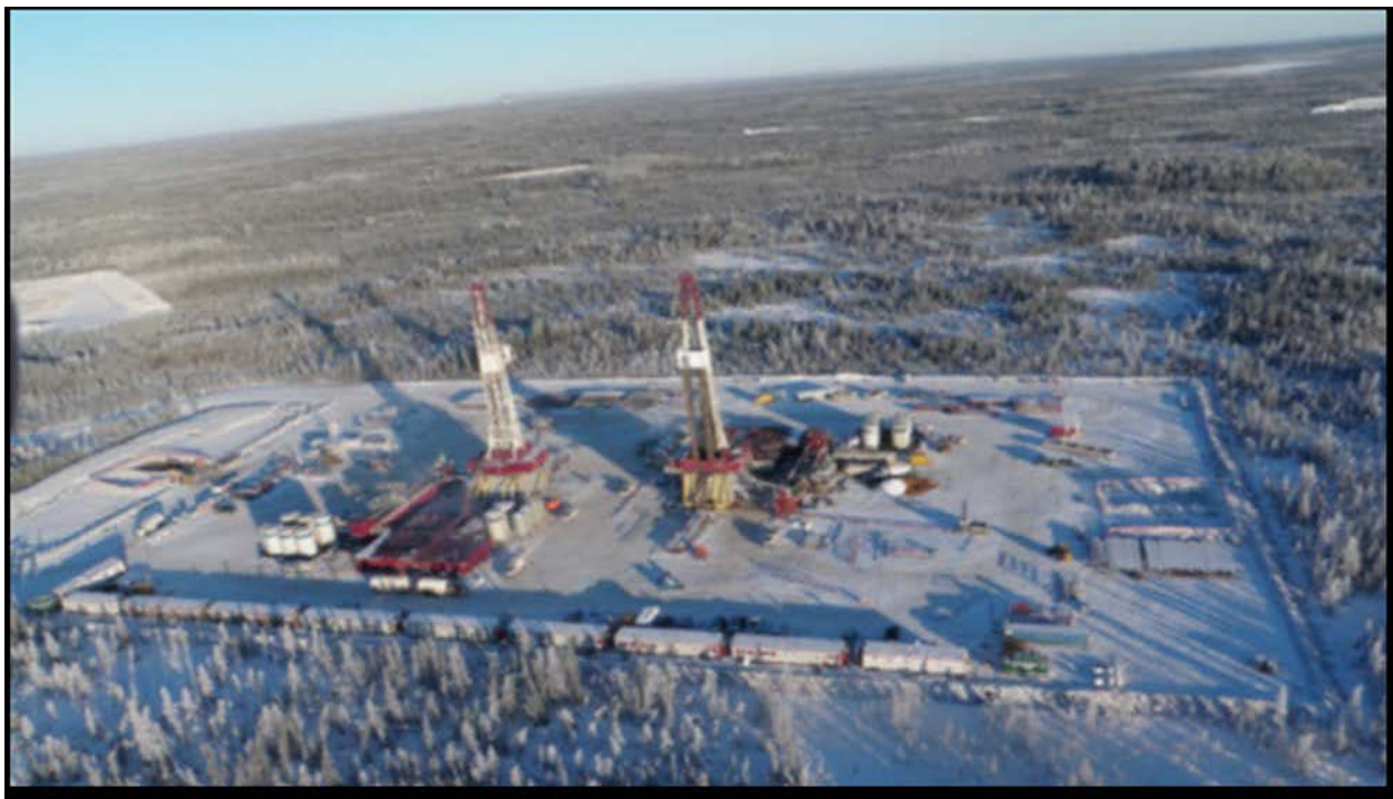
Figure 1: A hydraulic fracturing operation in B.C.'s Horn River using multiple wells on a single pad (Picture Courtesy of Nexen, 2010) 1 .
